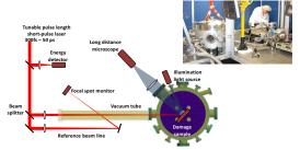
ARC optics are tested in the ARC damage test station.
